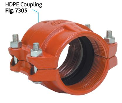
The Gruvlok Figure 7305 HDPE Coupling is a cost effective, easy to assemble, mechanical joint for HDPE pipe conforming to ASTM F714, D2447, D3000, or D3035 with wall thicknesses ranging from SDR 32.5 to SDR 7.3. The Gruvlok coupling method also eliminates the need for costly fusion equipment.
